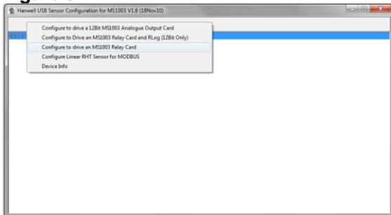
Fig 6 shows the config screen. Note its use should be self-explanatory. Select the alarm settings ensuring that this is done using the same scale and units as the RL5001 transmitter. Enter the MS1000 card ID and the Transmission Interval, see section 7 for further details.
