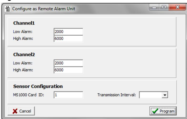
When the details are correct click on the “Program” button to save these settings into the Sensor.
